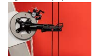
Knieelot mechanisch fernsteuerbar Remote mechanical adjustment of the knee position.
