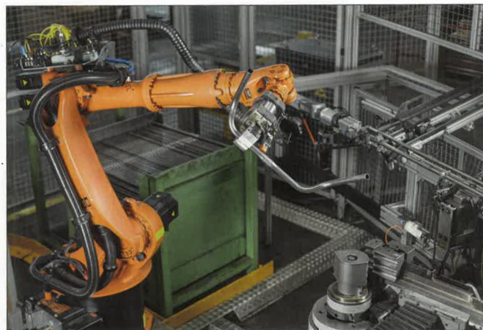
The bending of the tube is done fully automatically by Wafios bending machinery equipped with Kuka robots.
